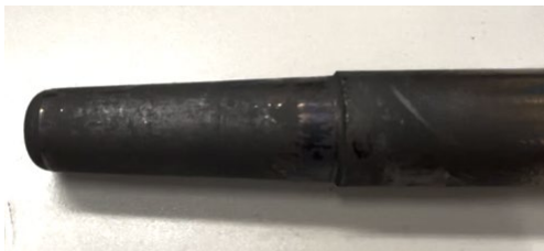
Figure 5. Photograph of one of the graphite coated core pins
