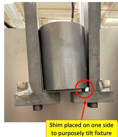
Figure 9. Photograph of the apparatus utilizing a shim to tilt the crucible by about 1.8 degrees.
