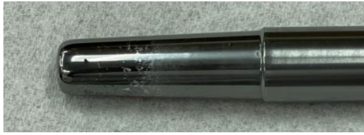
Figure 17. Photograph of the AlCrN coated pin after testing.
